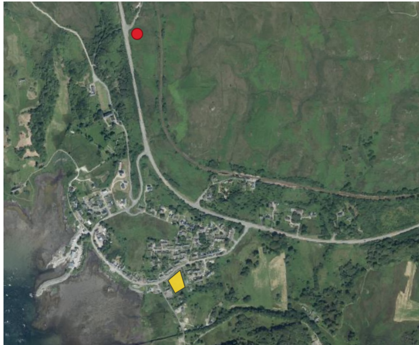
Figure 18: Scenario 1 assumed the installation of a 240kW solar array (yellow) and 100kW wind turbine (red) within Arisaig. The location of the solar array is for scale only and does not indicate any serious proposals to develop here.
